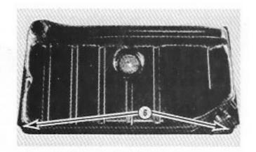
Bend the corners of the front fuel tank flange upwards as shown in photo.
