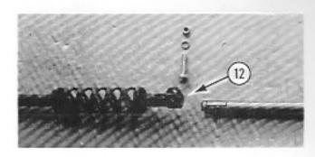
Remove the short VW steering shaft from VW rubber flex joint. Replace with the longer BCW steering shaft. Use the original VW hardened bolts, lock washers and nuts. After this connection is made, peen the ends of the bolts over the nuts as a safety precaution.
