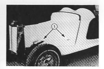
1 Insert the stem of the TD type hood handle through the factory pre-drilled holes in the hood side panels.
