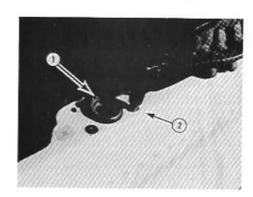
Attach hood release cable end to lower half of hood release and adjust cable through extra hole in side panel. When properly adjusted, the hood will automatically lock when closed.
