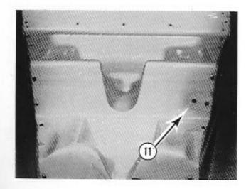
From the front of car, pass the BCW steering shaft through hole in front body section.
