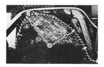
The rear portion of wiring loom is designed to follow the perimeter of the rear fender well. Attach loom wire ties to the inner fender well portion of the body side panel by drilling 1/8" holes and inserting 1/8" rivets as shown.
