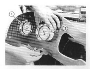
From underneath dash, drill 3/8" hole directly behind speedometer through cowl for speedometer cable. Insert new BCW speedometer cable through hole. Connect threaded end of cable to speedometer.
