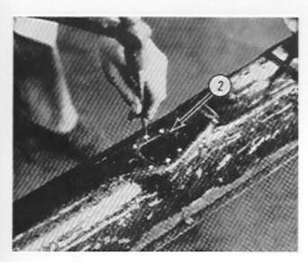
Scrape the paint and tar to expose the six spot welds under shifter plate. Center punch each of the spot welds.
