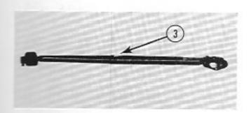
Align scribe line and weld or braze the end sections of the shift rod together.
