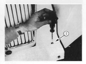
Attach splash apron to the front fenders with three chrome phillips head screws, one on the driver side and two on the passenger side. Secure with fender washers, lock washers and nuts.
