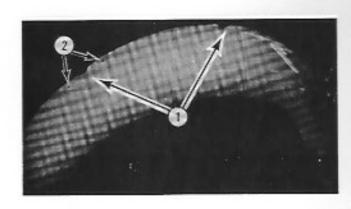
Align the factory pre-drilled holes and insert nine 1/4" X 3/4" carriage bolts through the underside of the fender to the interior of the car. Use fender washers, lock washers and nuts. Finger tighten only.
