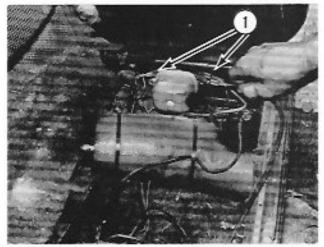
Remove the attachment screws and voltage regulator.
