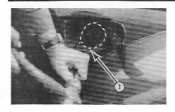
Using a cold chisel and hammer, cut sheet metal surrounding filler neck to remove from body.
