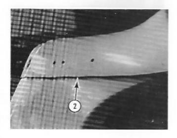
Check alignment on both sides. Properly installed, the cowl will have 1/4" off set from the body side panels.
