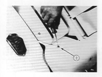
2 Insert chrome phillips head bolt through the factory pre-drilled holes in the splash apron and subframe.
