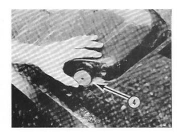
Plug original filler neck with 2" cut out saved from step (1) (previous page) and weld or braze closed.
