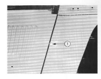
The gap between the hood side panel and the chrome radiator shell must also be even. Remember to check both sides of the car. Any necessary adjustments can be made by elongating the pre-drilled bolt holes (using a fine tooth, round file) and by shimming the mounting tab where it attaches to the cowl.
