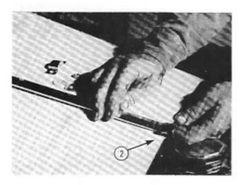
Install hood molding ends at each end of hood molding strip.
