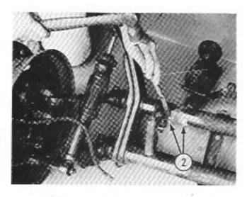
Using a cold chisel and hammer, remove factory locator tabs from the tube housing.
