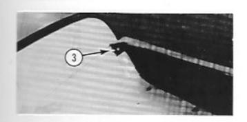
From passenger compartment insert 1/4" X 1" carriage bolt through cowl, front body section, and hood side panel mounting tab. Secure with lock washer and nut.
