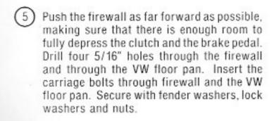
NOTE: To remove brake master cylinder or to adjust the brake extension, firewall must be removed.
