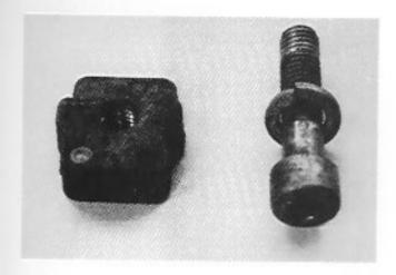
The upper end of the steering column assembly is attached to the steering column angle, underneath the dashboard and allen head bolts and rectangular nuts from the VW.
