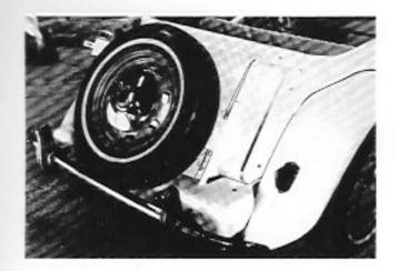
Mount the spare tire by placing the wheel over the factory installed studs on the carrier. Secure with the BCW wheel nuts.
