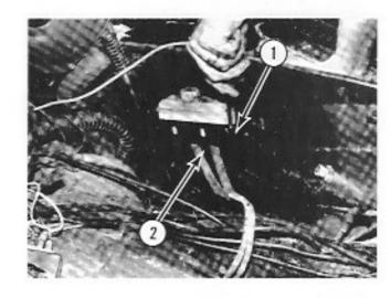
Disconnect reservoir lines from brake master cylinder and plug holes to keep out dirt.
