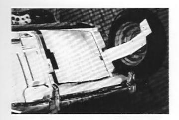
The all welded steel spare tire carrier is an authentic BCW detail that is a "look alike" reproduction of the original TD, engineered to fully support a real spare tire to swing to the side for easy engine accessibility.
