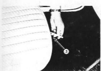
Place seat bottom on seat box. The rear portion of the seat bottom should fit underneath the seat back approximately 1".
