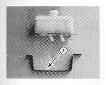
Bend metal strap to shape of VW brake fluid reservoir as shown.
