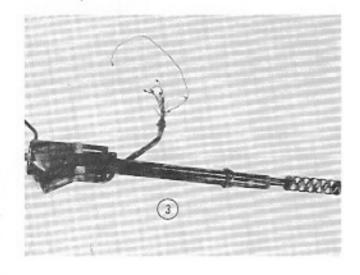
Remove steering column assembly from passenger compartment.
