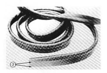
Apply contact adhesive to one side of the upholstery wind lace "flap" from the stitching to the edge. Be careful to keep adhesive off of bead.
