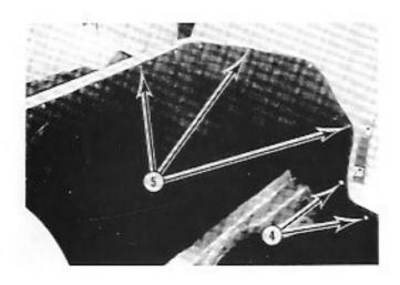
Glue carpet section #5 to center section using contact adhesive as in previous steps. Align top edge of carpet with wind lace bead. Glue carpet section #6 to firewall using contact adhesive as in previous steps.
