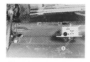
1 Place pedal relocation template\* on the driver's side of the tunnel and hold template in position with tape. The new pedal assembly location is 20" behind original position. Center punch all holes and drill according to template.
