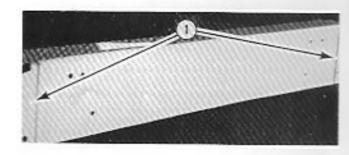
Insert four 1/4" X 3/4" carriage bolts from the outside of the body side panels through the side and rear body section. Secure with fender washers, lock washers and nuts.
