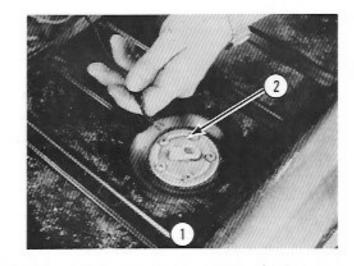
Remove filler and other hoses connected to the fuel tank.
