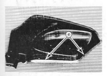
Using duct tape, seal edges.
