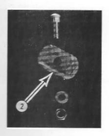
Attach side panel to chassis. Begin at the front of the car. Skip the first hole, then insert 5/16" X 1-1/4" large head carriage bolts down through the second, third, fourth, fifth, sixth and seventh holes. Place stock VW washers underneath the chassis, then a lock washer and nut.
