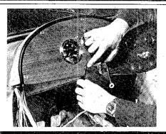
Center the dash in position so that the dash welting does not ride over the top of the dash cowl.
