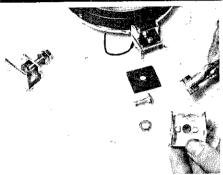
There are several places to mount fog or driving lights. We have found that the crank plate makes a good spot Set aside the portions of the light mount base you do not need, and make necessary modifications.
