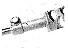
Drill a 5/32" hole completely through the column at the connection point of the rear shaft to the extension shaft. Install a compression pin and secure finally, with the original VW clamp.
