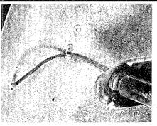
Find the mold mark on the crown of the front fender, set the rubber pad as far back as is possible and still cover the mark. Drill three ¼" holes. Feed the harness wiring up through the fender and into the lamp. Be careful not to scuff the harness in this lamp as the quarters are tight. If the mounting bolts are slightly too short, grind a little of the glass away under the fender.
