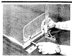
Lay the windshield frame on your bench slotted, or front edge, down. Set the wind wing on the frame and set the hinges parallel to the side. Slide the top hinge down  $3\frac{1}{2}$ " from the top and mark the frame through the hinge holes with a felt tip marker.
