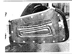
The doors have 14 finishing screws. When installed the washer or the screw should be at least 1/16" inside the nylon edge welting.
