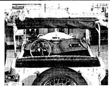
Pull the fabric from the front, through the bows, and wrap tightly around the bows.
