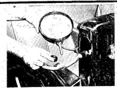
Drill a ¼" hole 1¾" directly back of the headlight tie-in bar. Install a rubber grommet (Note: Enlarge the hole with your rotary rasp, and cut your grommet to leave a tight fit.) Install the flex tube through the headlight shell hole, and insert the flex tube through the grommet. Paint the shell base black and install on top of the cradle. Install the shell mounting bolt through the base, the cradle, and secure with the provided nut.
