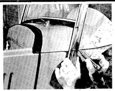
Place the frame into position on the body, make sure the bottom rubber extrusion is flipped forward, and push the windshield down until you measure 13¼" or less from the underside of the top frame member to the dash cowl, at the edge.
