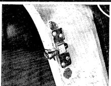
With your cone shaped rotary rasp, neatly remove enough of the door jamb to allow the striker to lie flat Engage the striker to the latch.
