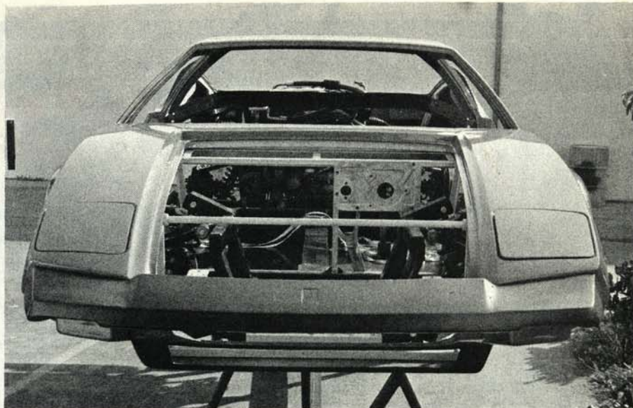
Inner steel subframes surround the occupants and strengthen the body.
