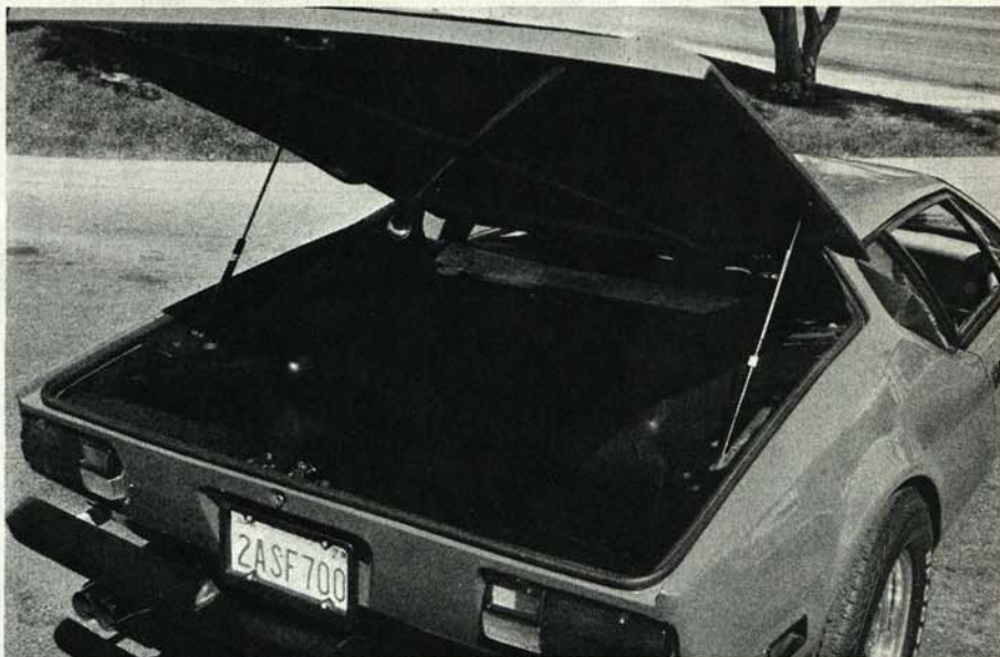
The gas and oil are serviced under the trunk.
